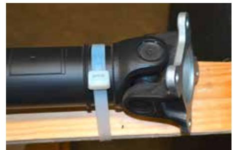
Lay the on-board strapped shaft into the box. Fill it with the formerly contained filling material and seal the box. Send the shaft back in accordance with the existing core-return-criteria to the core-and warranty center.
