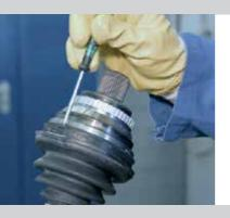
Fill 2/3 of the grease provided in the repair kit into the boot and the remaining grease into the joint.
