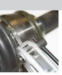
Endless retaining clips part no. 190136 (Content: 25 pieces)
