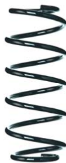
CC shaped spring – spring ends have different diameters so care is needed when fitting!
